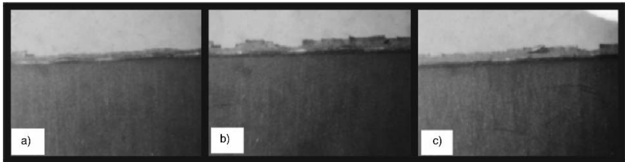
Fig. 11 Adhesion tests of AISI 4340 Zn-Ni-electroplated alloy coatings. (a) 2 to 6 \mu\text{m} . (b) 7 to 12 \mu\text{m} . (c) 15 to 21 \mu\text{m}
